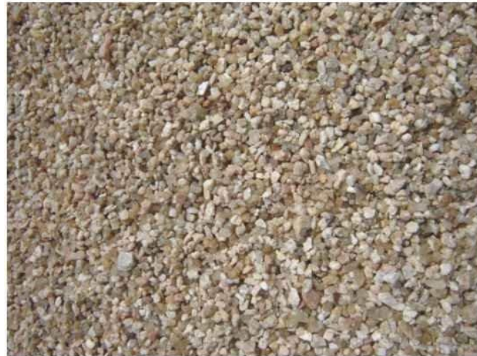
FILTER MEDIA SAND CLEANED & GRADEDS SIZES .5mm -1.2mm & 1.2mm-2.4mm
