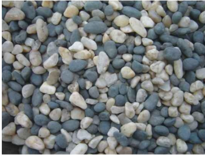
FILTER MEDIA STONES WASHED & GRADED 2.5-6.5mm, 6.5-10mm, 11-25mm & 26-50mm
